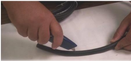
Figure 4.12 Strip the outer jacket
