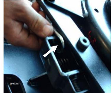
Figure 5.7 Padlock into Eight o'clock position
