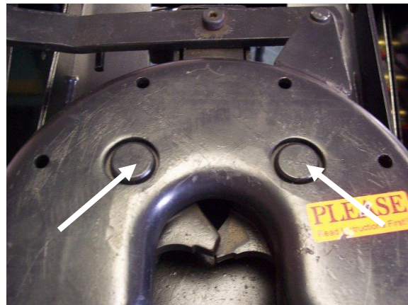
Figure 6.4 Jaw Pivot pins location
