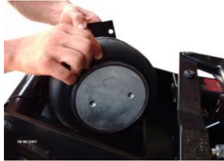
Figure 4.4 Airbag placement (PN 45550)
