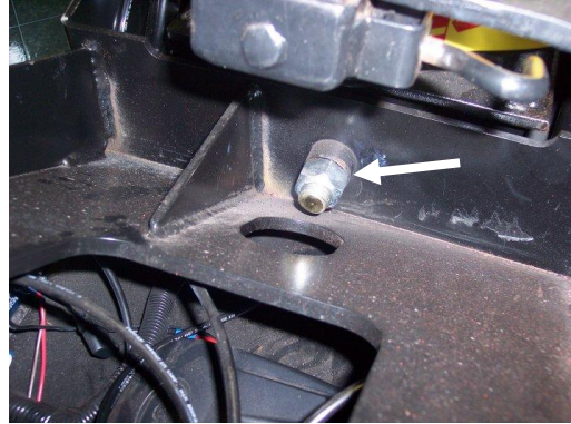
Figure 6.2 Check pivot bolt wear (PN 44031)
