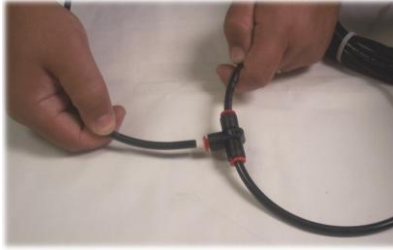
Figure 4.14 Insert into tee fitting (PN 49212)
