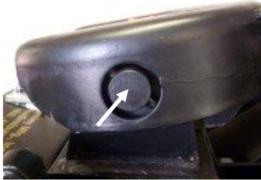
Figure 7.1 Lubricate fore and aft pivot pins
